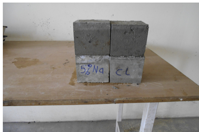
Fig. 6. Visual observation of GPC3 exposed to 5% NaCl solution for 90 d.
