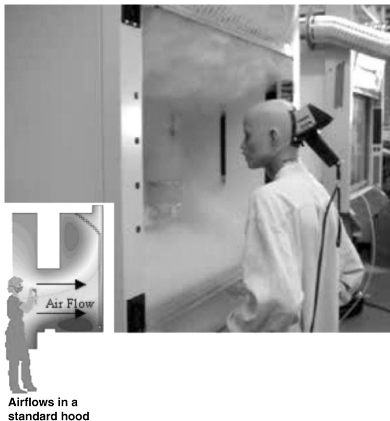
Fig. 3. High-performance laboratory fume hoods. In a conventional laboratory fume hood, air is drawn past the worker and exhausted through the top of the hood. Workers and experimental apparatus can interfere with airflows and thereby cause dangerous eddies and vortices (red and blue circular areas in the inset) with potential for fume spillage and hazards to workers. The Berkeley Hood (shown in photo) instead utilizes a curtain of air introduced from above and below the hood opening in front of the worker, with up to 70% reductions in airflow (and corresponding energy savings) and improved worker safety as a result (Bell et al., 2001).
