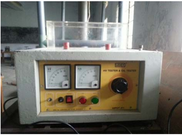
Fig. 2. Image of High Voltage oil Tester (model OTS-E) for breakdown measurement.
