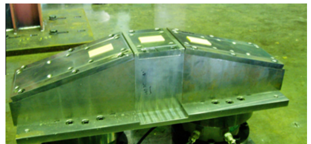
Fig. 4. Lower component of the test specimen with PTFE pads.
