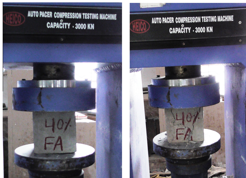
Fig. 5. Compression test (before and after test).
