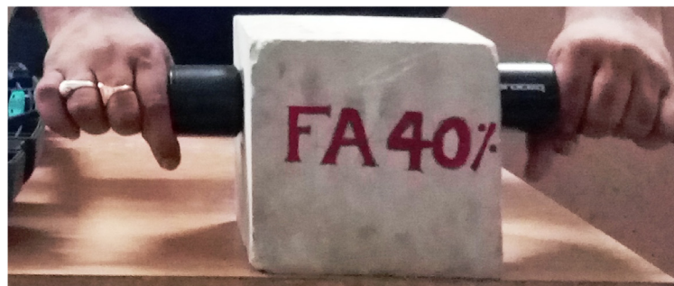
(b) UPV Test on Cube Specimen
