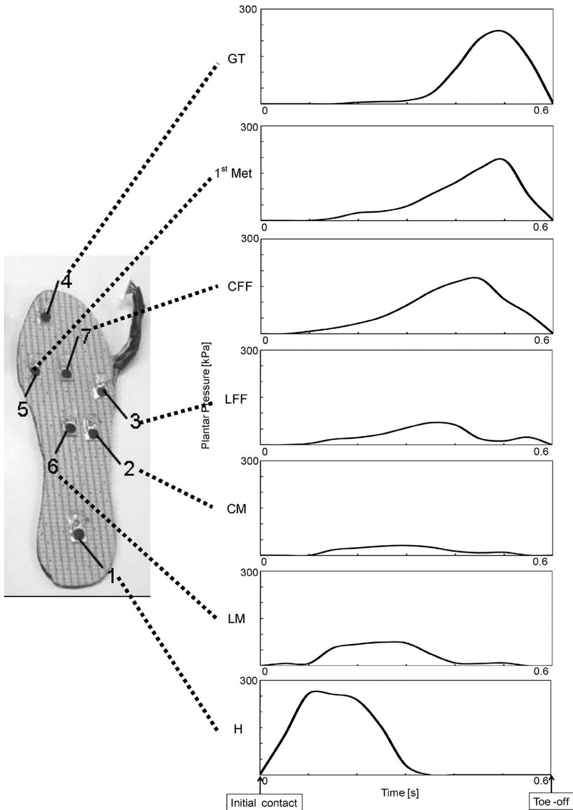
**Fig. 6.** Pressure patterns recorded by an individual's sensors during a step. The data are the same as those shown in Fig. 5. The pressure patterns for the right foot have been magnified and separated by sensor for clarification.
