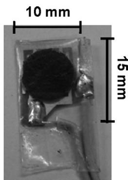
Fig. 1. A pressure-sensitive conductive rubber sensor (PSCR sensor) that was used to measure plantar pressure.
