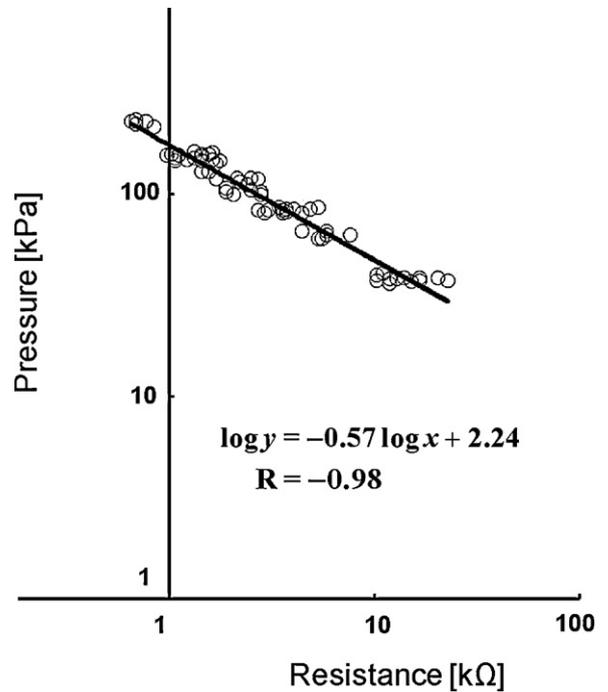
Fig. 2. The relationship between pressure and rubber resistance.
