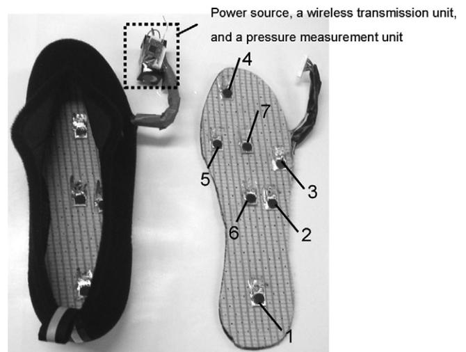
Fig. 3. All-in-one in-shoe device developed to measure plantar pressure. Sensors were placed at seven locations: heel (sensor #1, H), lateral midfoot (#2, LM), lateral forefoot (#3, LFF), great toe (#4, GT), head of first metatarsal (#5, 1st Met), centre midfoot (#6, CM), and centre forefoot (#7, CFF).
