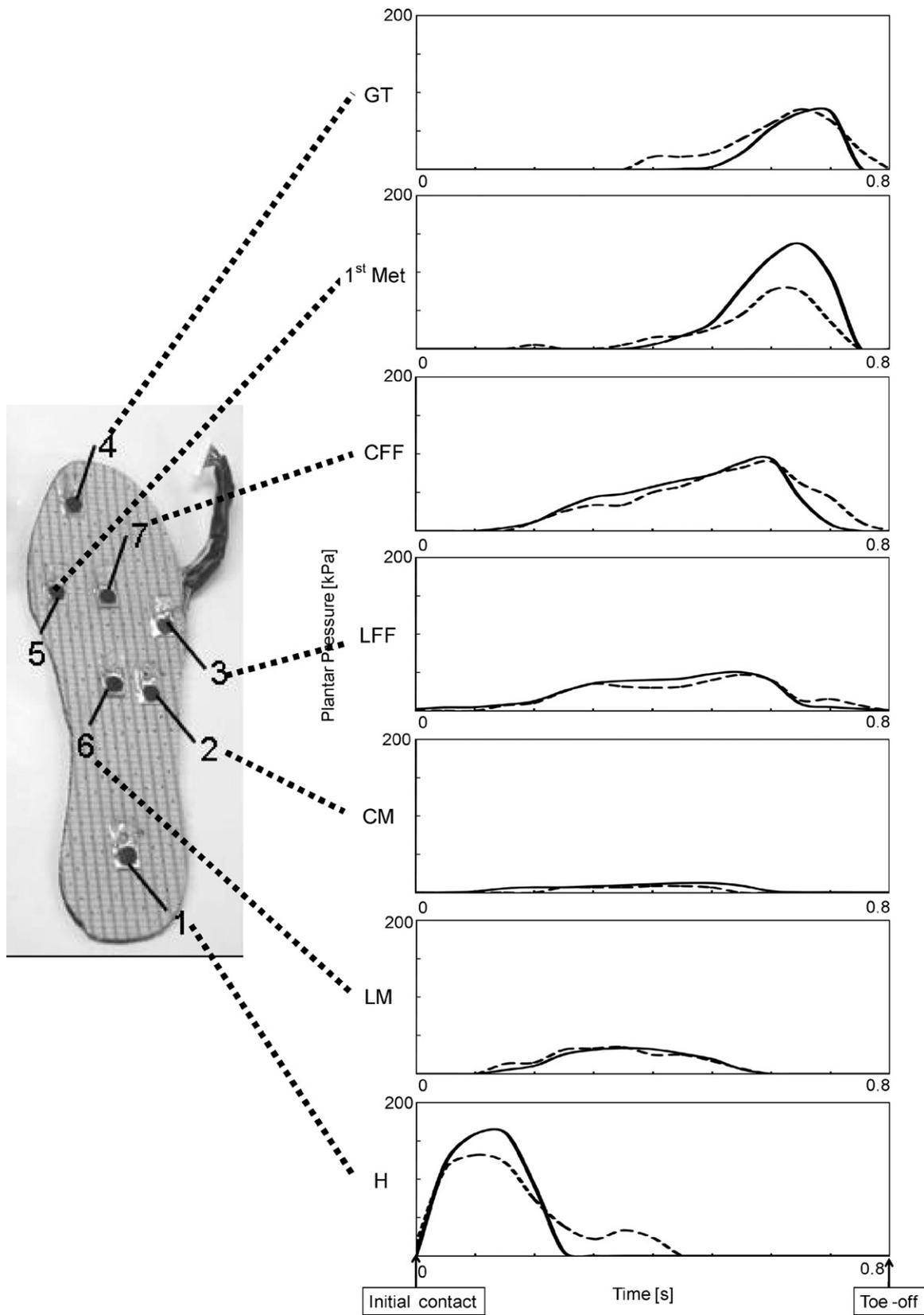
Fig. 4. Pressure patterns obtained from our device and a F-scan system placed on the right foot during a step in a healthy 25-year-old subject.
