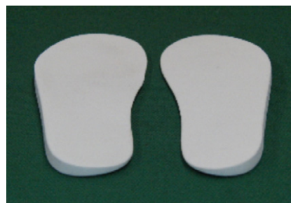
Fig. 1. Laterally wedged insoles used in this study. These ethylene vinyl acetate insoles had an 8^\circ posting along the entire lateral border.
