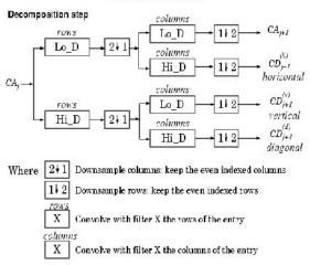
Fig 2: Decomposition Steps in 2-D DWT
