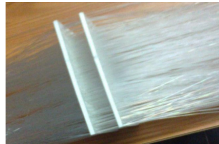
Fig 3. Optical Fibres running through 2 perforated sheetings.
