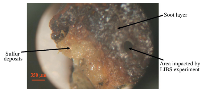
Fig. 10. Sulfur/soot deposits collected from the combustion of \text{H}_2\text{S}/\text{O}_2/\text{C}_3\text{H}_8 .
