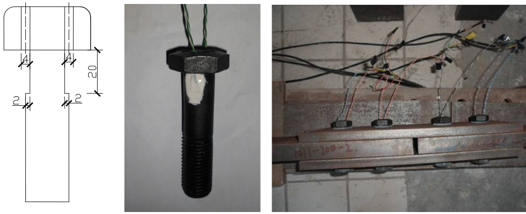
Fig. 2. Layout of strain gauges on the bolt.
