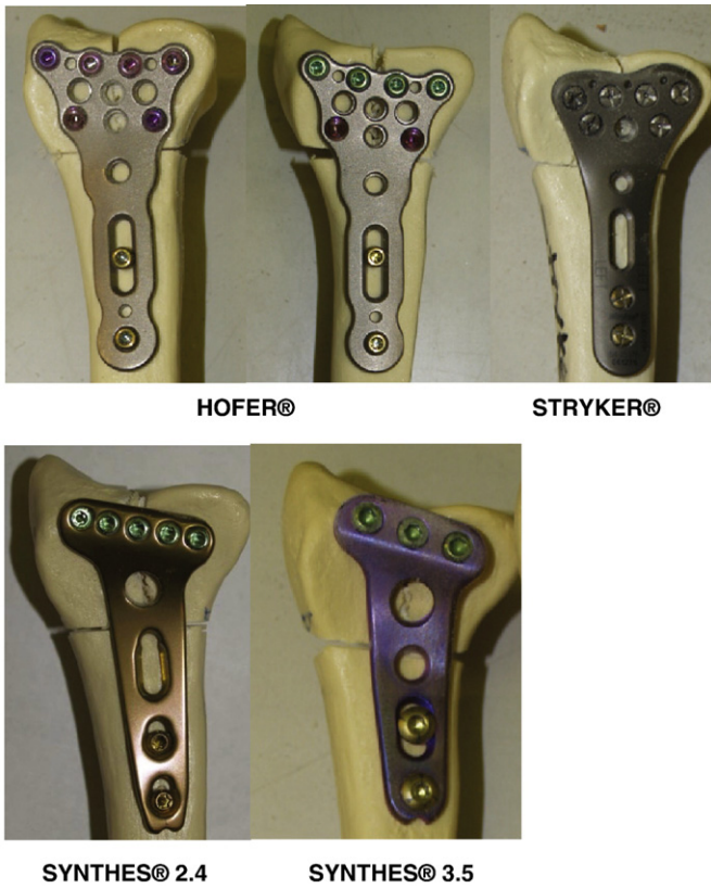
Fig. 1. Sample-types; two implants of the same type with different screw-realisation were tested in case of Hofer®.
