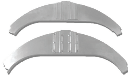
Fig. 4. Structural aerospace assembled component as the proposal part machined in one step [7].
