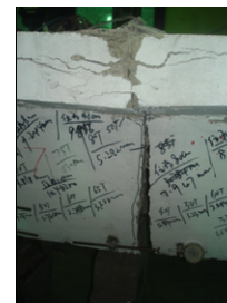
(f) failure due to concrete
