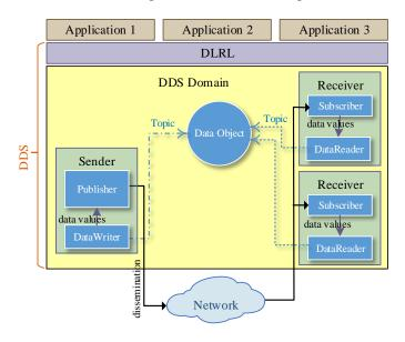
Fig. 16. The conceptual model of DDS.
