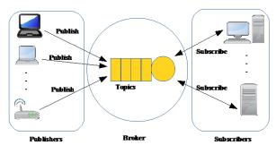
Fig. 8. The architecture of MQTT.
