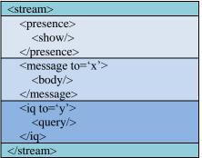
Fig. 12. Structure of XMPP stanza.
