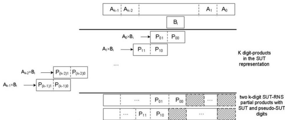
**Fig. 5** Rotating digit products resulted from multiplying  $B_i$  by  $A$ , and producing two final partial products in Stage 3
