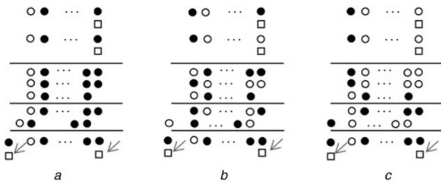
Fig. 7 Notations of three existing digit-products additions for modulo  $2^n + 1$  addition tree in stage 4
