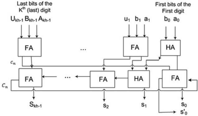
**Fig. 2** Redundant end-around-carry adder for two  $k$ -digit modulo  $2^n - 1$  SUT-RNS residues
