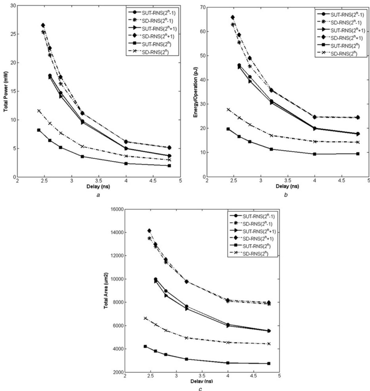
**Fig. 8** Synthesis results of SD-RNS and radix-8 SUT-RNS multipliers for moduli set  $\{2^6 - 1, 2^6, 2^6 + 1\}$  against different delays
