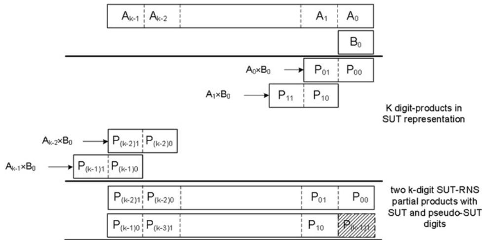
**Fig. 4** Rotating digit products resulted from multiplying  $B_0$  by  $A$  and producing two final partial products in Stage 3
