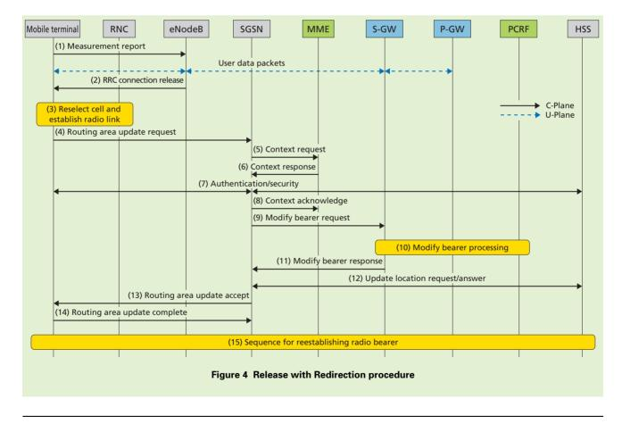
switches the communications path to the SGSN and returns a modify bearer response message to the SGSN.
