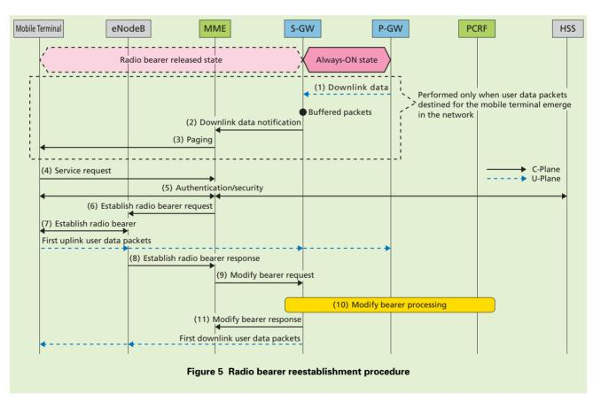
tion and security-related procedures, the MME sends an establish radio bearer request including the S-GW IP address and bearer information to the eNodeB.
