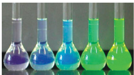
Figure 5. Photograph of CdSe/CdS CS NCs with core sizes ranging from 1.2 to 1.5 nm, exhibiting PL Q.Y.s of 60–80% (under room light). Reproduced with permission from Reference [51].
