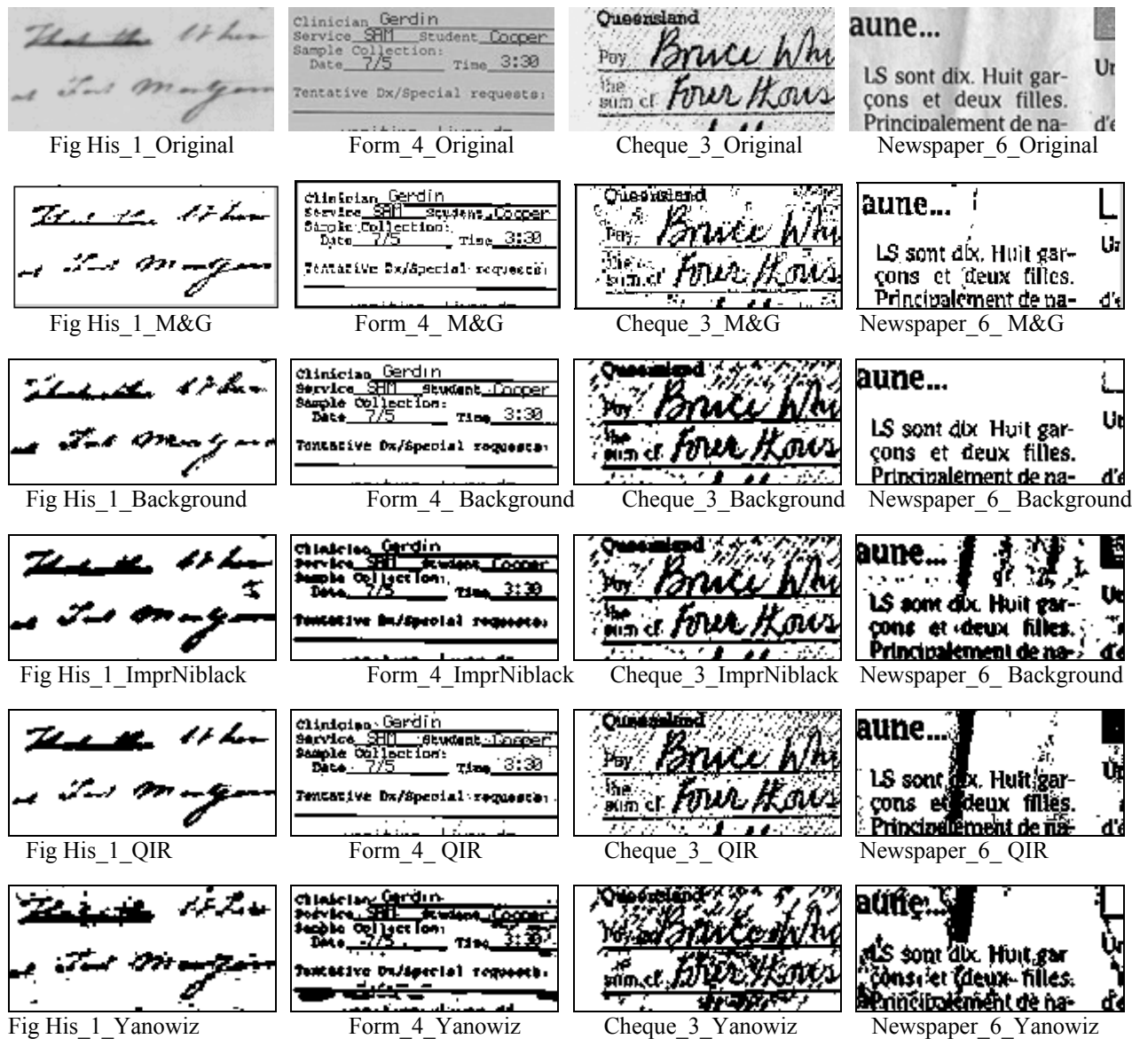
Figure 1. Examples of sections of part of each of one of the four types of 'difficult' image under investigation and the result of the five threshold methods described.
