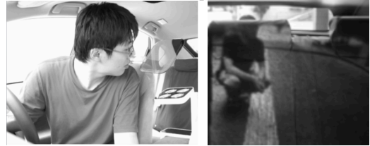
Figure 3. (Left) Driver's experience: driver was able to see image (Right) which was captured by the cameras behind the car.
